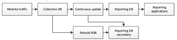
This diagram shows the processing required to rebuild the entire reporting database on request.
